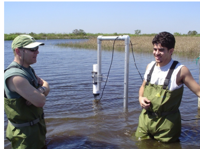
Installing an Acoustic Doppler Velocity Meter in the Everglades
